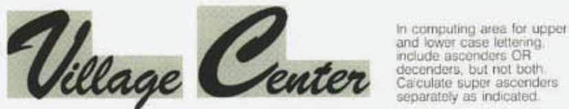
Figure 1003.4 SIGN AREA - COMPUTATION METHODOLOGY Sum of Shaded Areas Only Represent Sign Area for Code Compliance Purposes Signs consisting of individual letters, elements, or logos placed on building walls or structures
